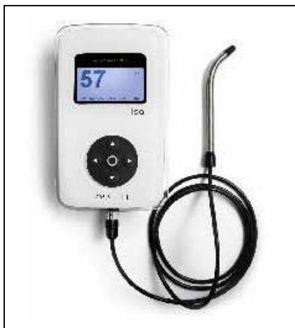
Figure 3. Osstell ISQ Instrument.
