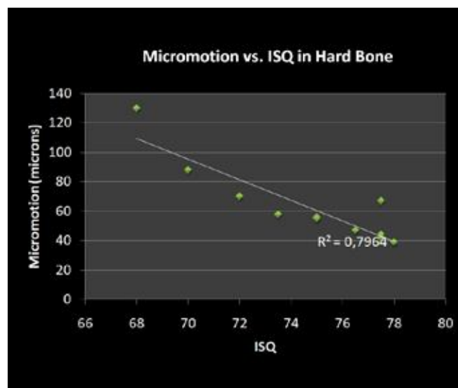
Figure 6. In the Hard bone, regression analysis and Spearman's rank correlation coefficient shows a high dependence between all values of the micromotion and the ISQ values, indicating that micromotion decreased with increasing ISQ values \rho=-0.89 r^2=0.80 P=0.0002 ; the variables are correlated and test is statistically significant.
